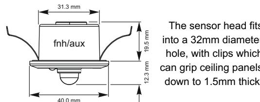
The sensor head fits into a 32mm diameter hole, with clips which can grip ceiling panels down to 1.5mm thick.
