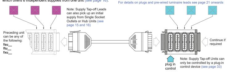
Supply Tap-off Leads are available in 3 or 4 core depending on whether an emergency test is required locally on each unit, or globally across one unit to the next
