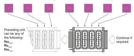
Note: All luminaires will be controlled as one. If using a plug-in control device it can be plugged into any spare outlet on the run. For details on plug-in control devices see page 33
