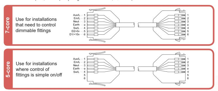
\* Plastic flexible conduit is 16mmØ black. It contains the appropriate number of loose single cores in LSHF at the csa indicated by the part number.
