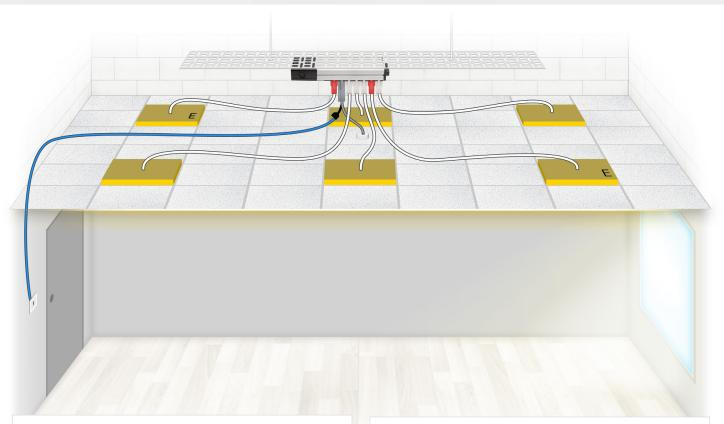
Control of the luminaires is via a flex7 plug-in sensor head and switch, both operating at PELV. The luminaires are manually switched on with a short pulse of the switch, after which they remain on whilst movement is sensed. After the room is vacated the luminaires switch off when the timeout period has elapsed.
