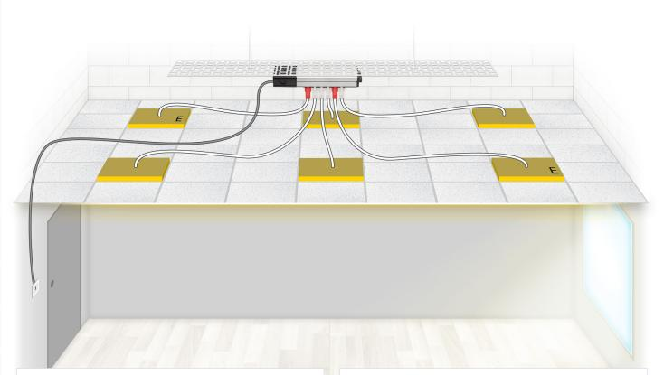
Control of the luminaires is from 1 location via a traditionally hard-wired 230V, 1-way switch; a small range of 230V plug-in switch drops are available if preferred.
