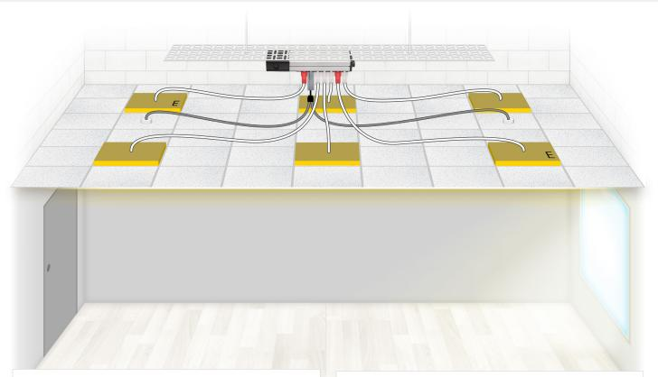
Control of the luminaires is via 2 flex7 plug-in sensor heads operating at PELV. The luminaires are automatically switched on when movement is sensed. After the room is vacated the luminaires switch off when the timeout period has elapsed.
