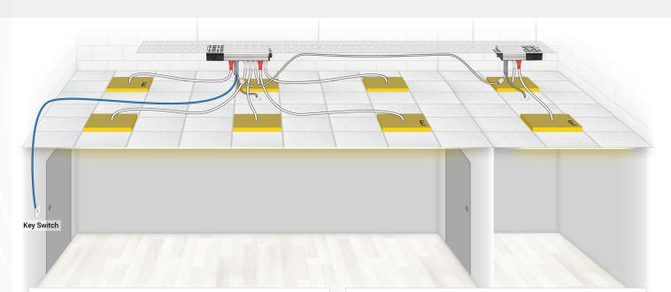
An Office and adjoining Store Cupboard, each protected by different devices at the distribution board (could be different phases), requiring individual occupancy control, but a single key switch to facilitate emergency test across both circuits.
