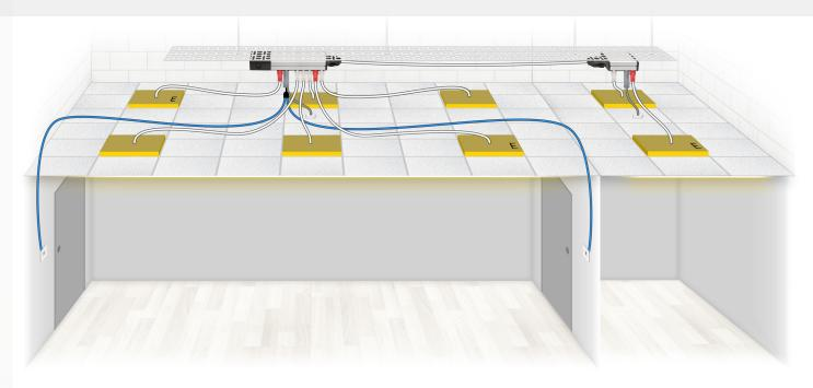
Originally 1 large office. Reconfigured to create 2 separate spaces, requiring individual control; absence for the Office; occupancy for the Store Cupboard.
