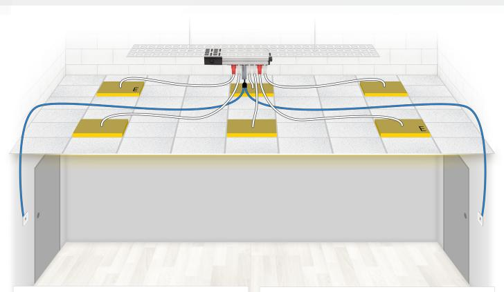
Control of the luminaires is from 2 locations via flex7 plug-in switches operating at PELV. The luminaires are manually switched on or off with a short pulse of either of the switches.
