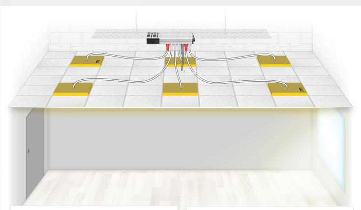
Control of the luminaires is via a flex7 plug-in sensor head operating at PELV. The luminaires are automatically switched on when movement is sensed. After the room is vacated the luminaires switch off when the timeout period has elapsed.
