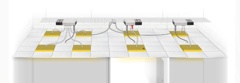
Two Offices, either side of a central Corridor, all protected by different devices at the distribution board (could be different phases); all three requiring individual occupancy control.
