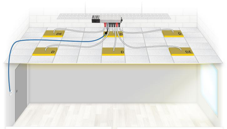
Control of the luminaires, both switching and manual dimming, is from 1 location via a flex7 plug-in switch operating at PELV. The luminaires are manually switched on or off with a short pulse of the switch. Once on, the luminaires can be dimmed or brightened by holding the switch until the desired light level is reached.
