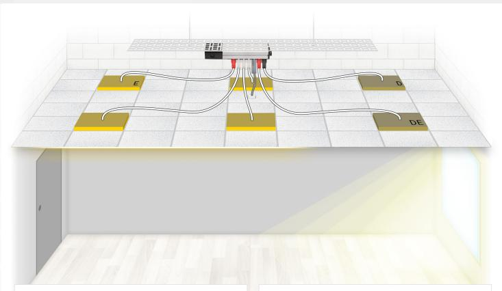
Control of the luminaires is via a flex7 plug-in sensor head operating at PELV. The 2 luminaires adjacent to the window are dimmable.
