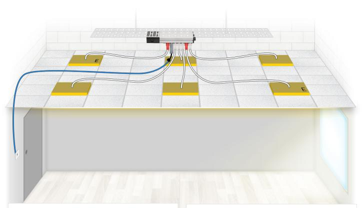
Control of the luminaires is from 1 location via a flex7 plug-in switch operating at PELV. The luminaires are manually switched on or off with a short pulse of the switch.
