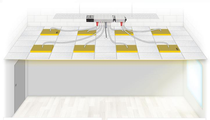
2 of the luminaires have been added at a later date to the original 6, resulting in the Distribution Box being too small for the new layout. A flex7 Expansion Box is plugged directly into the end-cap socket of the original box, instantly increasing the number of available outlets. The 2 boxes now operate as 1. A range of expansion leads are available if the installation would benefit from the 2 boxes being remote from each other.
