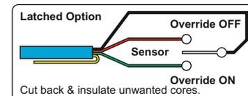
**Note:** Alternative operational options not necessarily shown above are available using the **frc/set** setup remote control.
