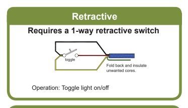
Retractive switching is ideal for multiple switch points. Just plug in any additional switch drop/s alongside the existing using our standard 'Y' adaptors.
