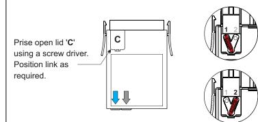
Lights can remain ON during an emergency test. Wire connection unit as shown on page 5.
