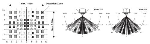
The X-Y cross-sectional diagram shows the detection area. The differences in the detection zone patterns indicate the projections of the 16 lenses with a single focal point. Movement of an object with higher than background temperature, between the detection zones, will be detected.
