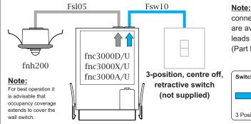
Note: Multiple switches can be connected in parallel. 'Y' connectors are available to enable two switch drop leads to be connected into one point. (Part No. fsy/A - adaptor)
