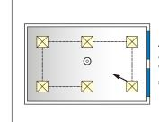
As lamp output across the circuit must be common, it is not possible to provide the 'optimal' ON/OFF state for all areas when some receive more daylight than others.
