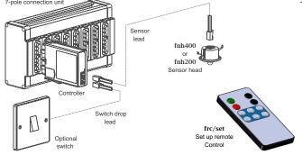
The frc/user remote control is a convenient method for the user to control the lighting remotely.
